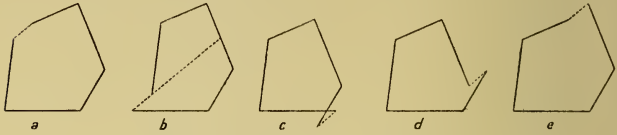
FIG. 157.—Closing Error of a Polygon.
